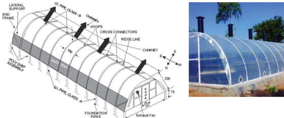
**Figure 6.** Walk-in type hemi-cylindrical solar tunnel dryer (Rathor and Panwar, 2010).
