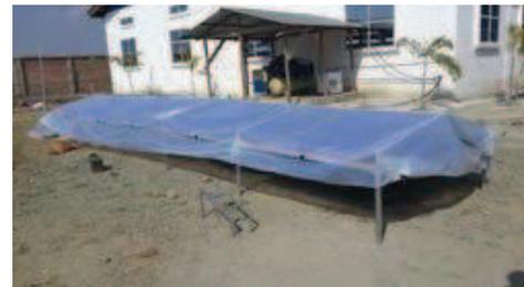
Figure 5. Schematic diagram and photo of solar tunnel dryer (Bala and Janjai, 2009).
